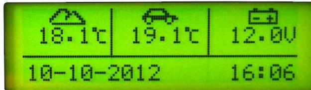
Temperature screen also displays the date and current time. If you connect the signaling state of the radiator fan, his work is indicated in the form of changing the third icon (thermometer / fan). You can also switch to battery (accu) voltage measure (SW2) in third window.
