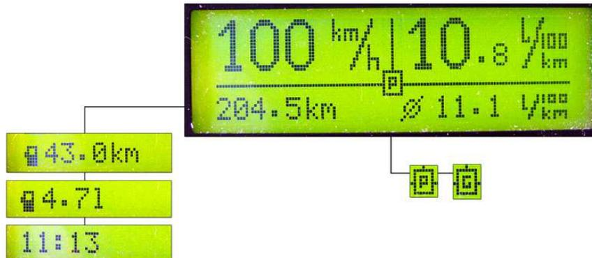
All these options are counted and stored separately for two types of fuel, ie. instantaneous and average fuel consumption will be different for petrol and gas (the same with distance or amount of fuel in the tank). In the UTCOMP settings you can enter another injection constant for PB and another for LPG (usually a constant injection for LPG will be about 10-20% greater than the constant injection for the PB).
