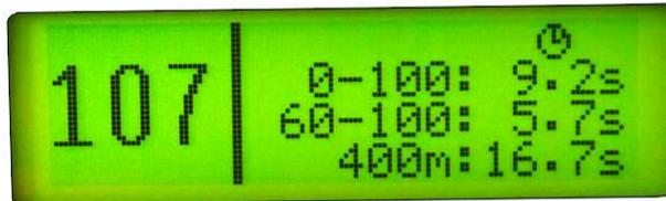
The screen displays the currently set intervals, and current speed measurements. Refreshing parameters on the screen are slower and less accurate than measurement procedure.
